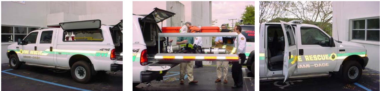
Example of extended cab 4WD Pickup with pullout equipment tray (courtesy FL-TF1).
